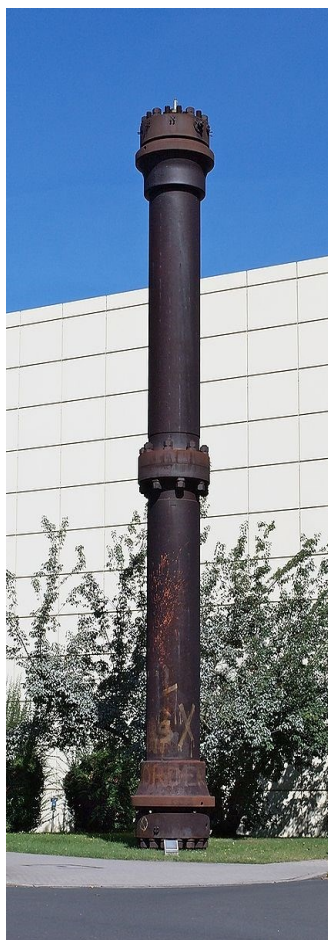
Historical first pressure steel reactor used for ammonia production by Haber in 1921
